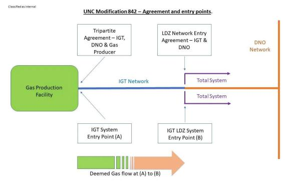
The proposed 'operator to operator' agreement at the physical interface between gas producer and Pipeline as proposed by UNC Mod 0842
